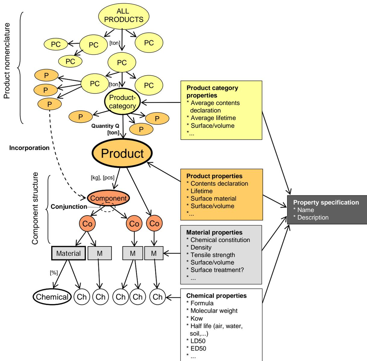
Figure 8 The concepts related to products in Chemitecs concept model: from chemicals via material, components, product to product categories.
