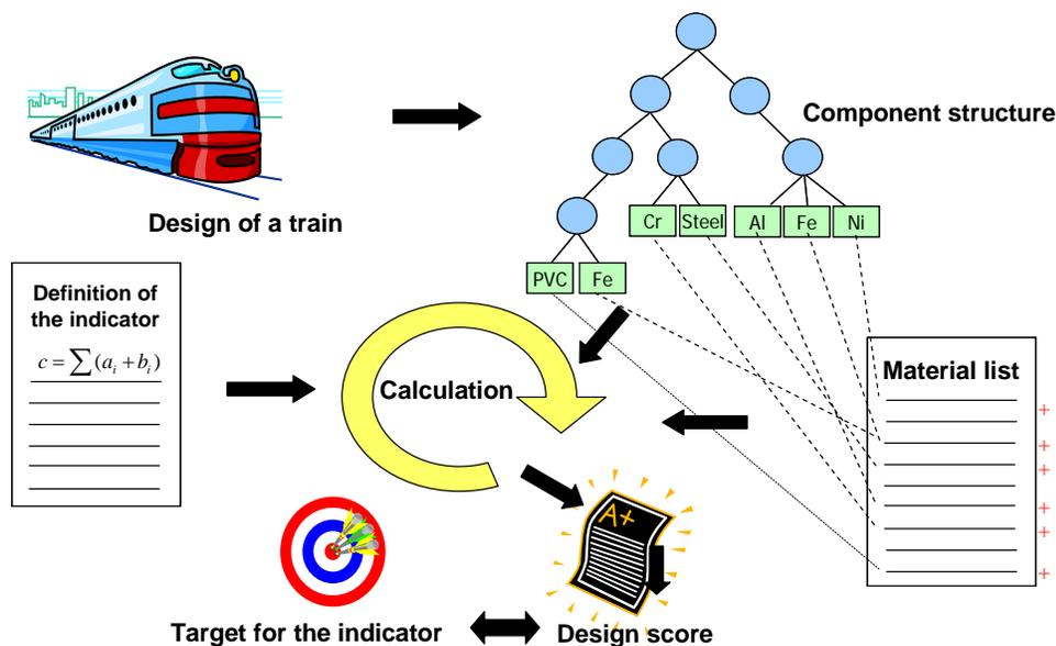
Figure 5 Conceptual approach from the RAVEL project for calculation of Environmental Performance Indicators of product designs (Carlson, Forsberg, 2000).
